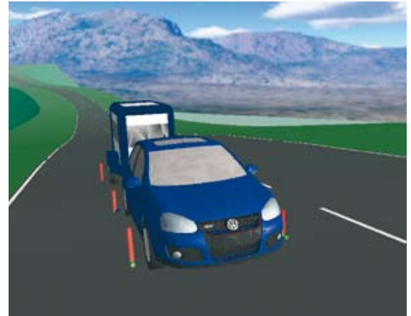
Virtual stabilisation tests of the vehicle-trailer combination with CarMaker/HIL – example of the new ESP system's performance tests.
