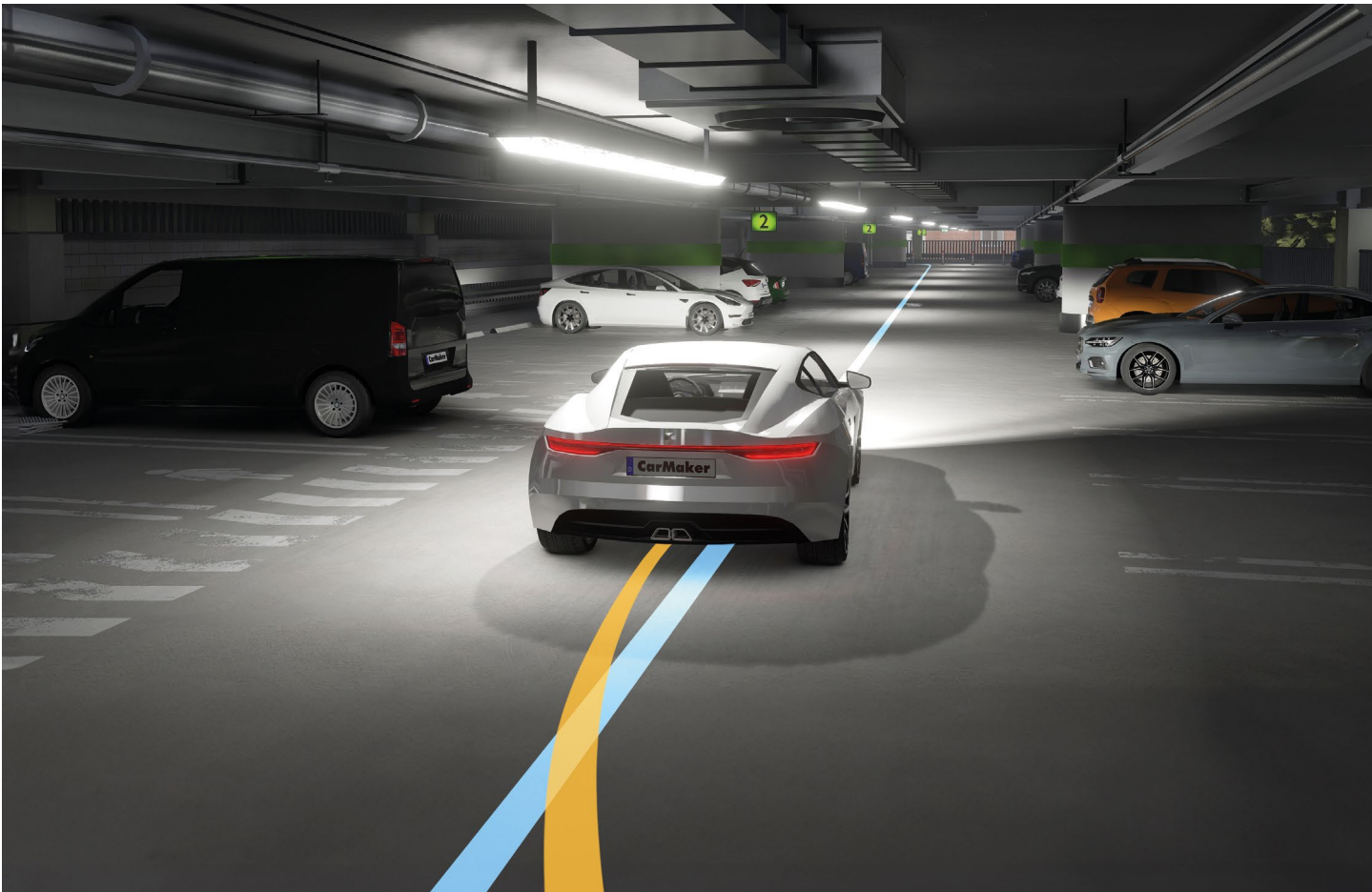
FIGURE 3 Scenario in the parking garage: predefined trajectory (blue) and the trajectory actually traveled by the ego vehicle (orange) (© Technical University of Darmstadt, IPG Automotive GmbH)
