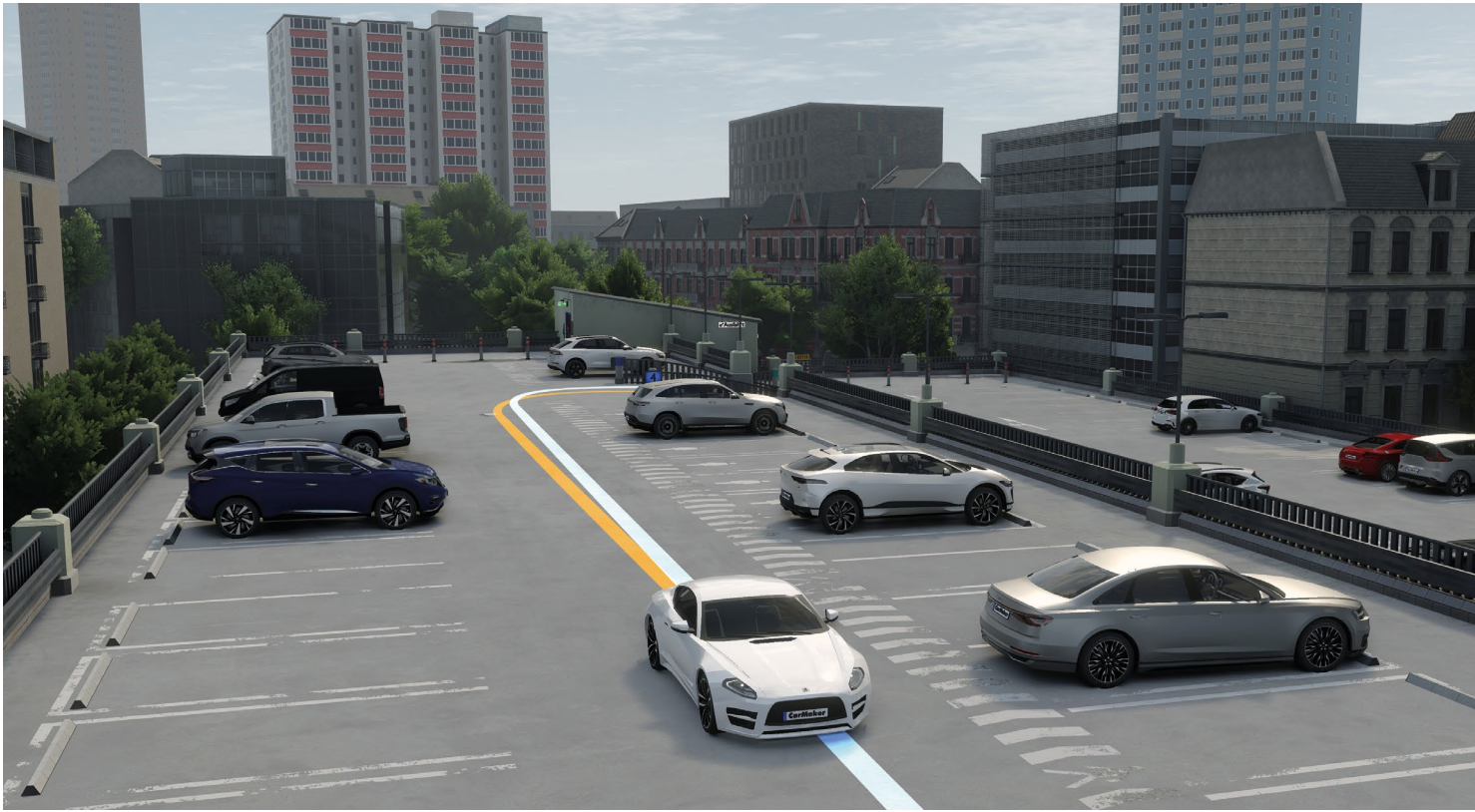
FIGURE 4 Test scenario in a parking garage including the trajectory traveled by the ego vehicle (white) (© Technical University of Darmstadt, IPG Automotive GmbH)
