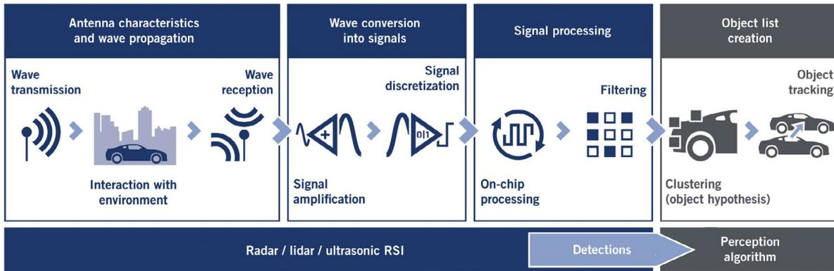
FIGURE 1 Signal chain of the RSI sensor models (© IPG Automotive)
