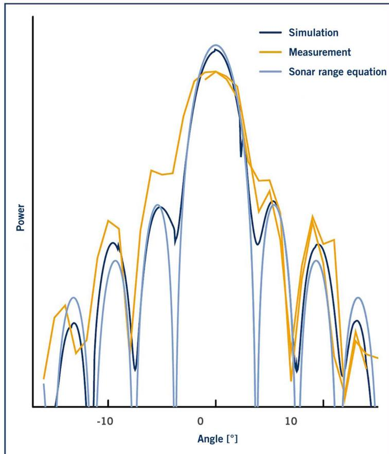
**FIGURE 4** Results of the test "turnable plate" and comparison with the data calculated in simulation (schematically) (© Continental | IPG Automotive)
