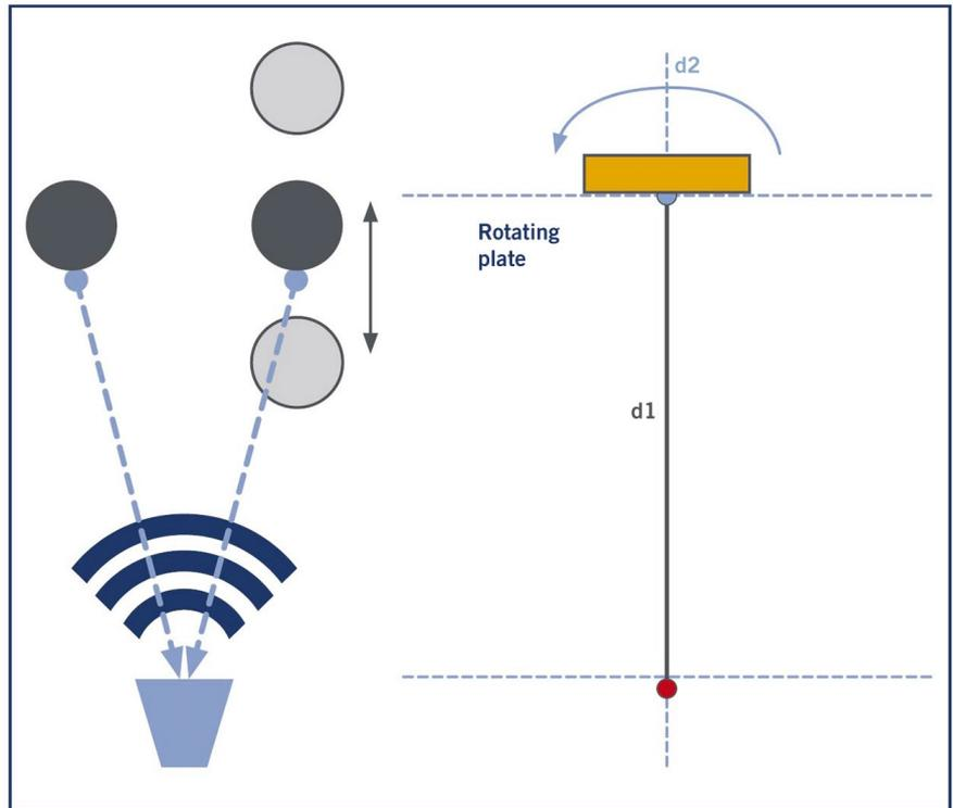
**FIGURE 3** Test setup A (left) and B (right) to validate the sensor model Ultrasonic RSI (© Continental | IPG Automotive)
