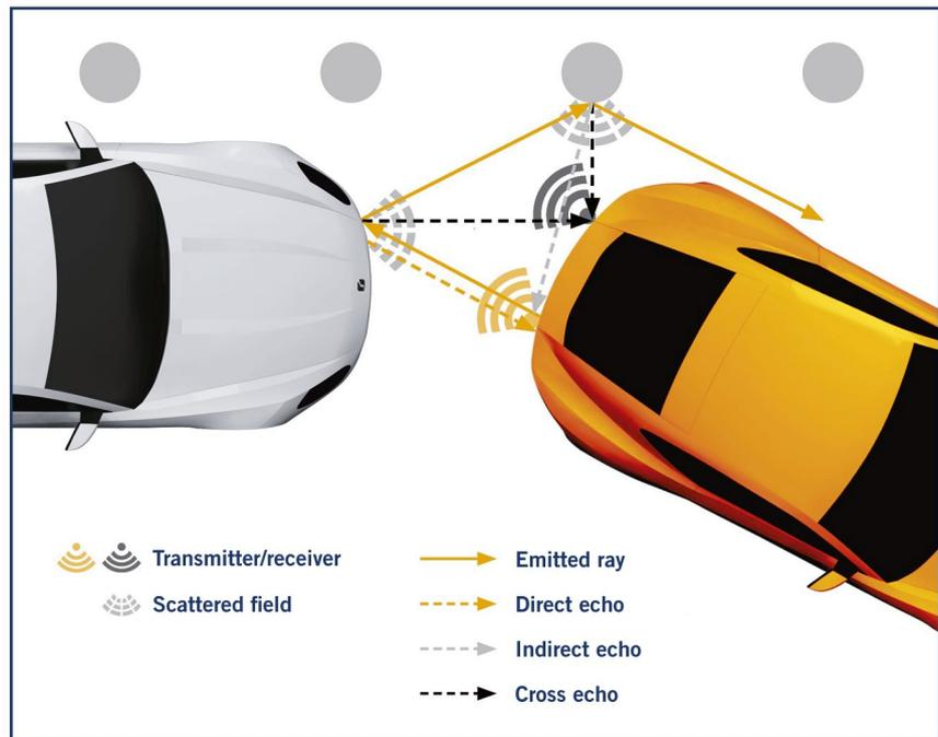
FIGURE 2 Schematic representation of the ray tracing algorithm to simulate a sound wave (© IPG Automotive)
