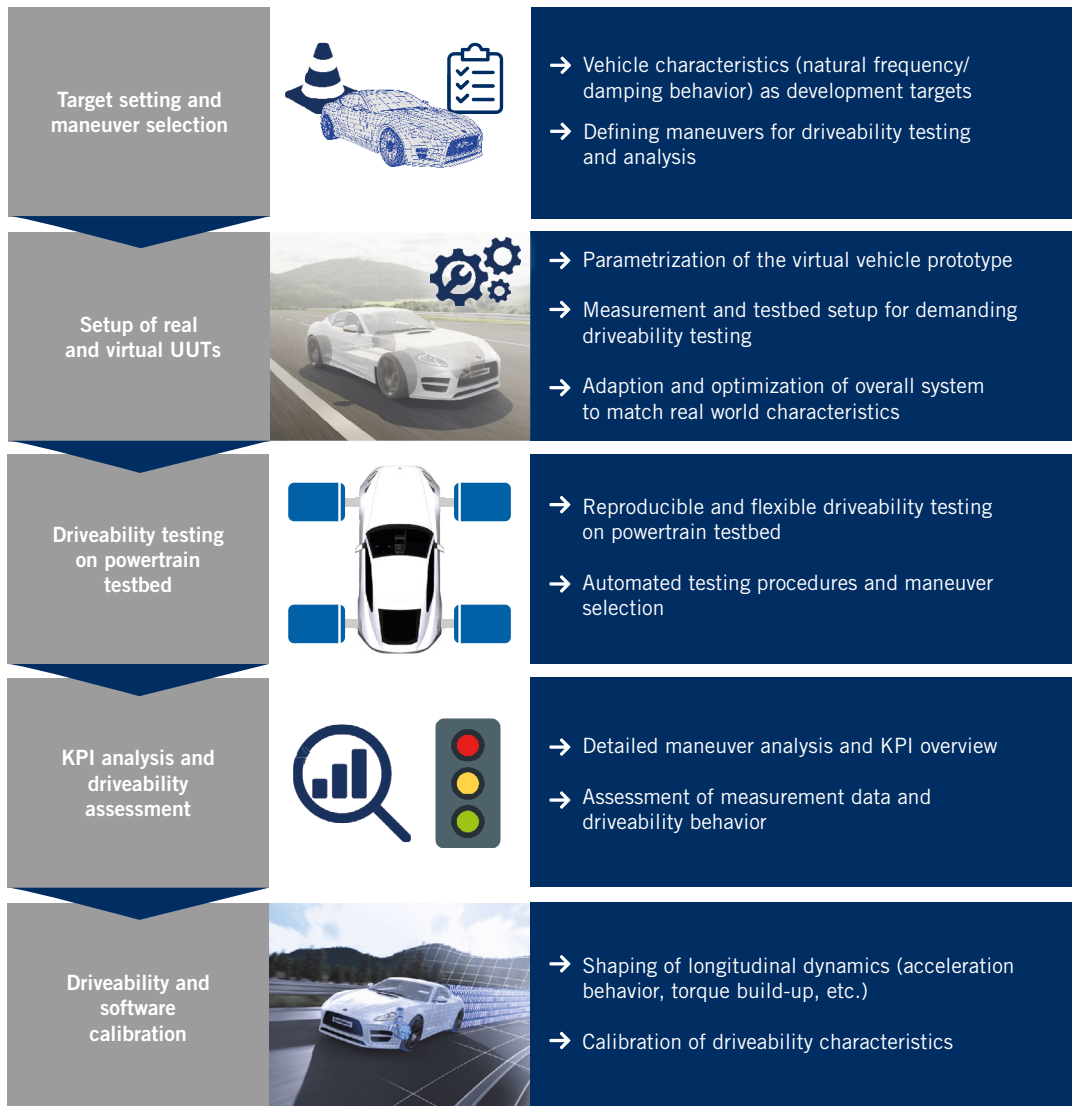
FIGURE 5 Method for developing driveability on a dynamometer (© IPG Automotive)
