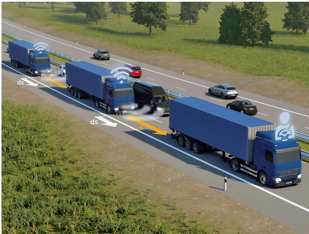
FIGURE 1 Platoon vehicles in the simulation environment TruckMaker (© IPG Automotive)
